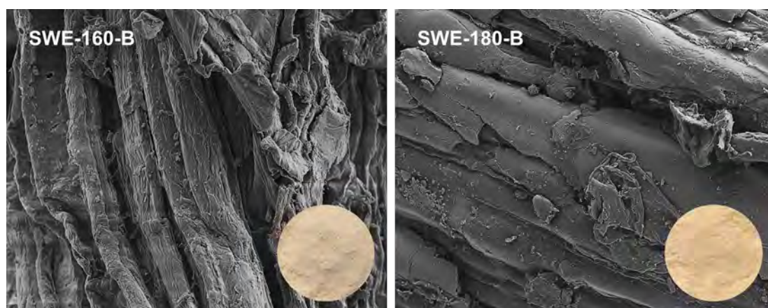
Fig.1 FESEM images of the bleached fibres (X 2000) and visual image.
