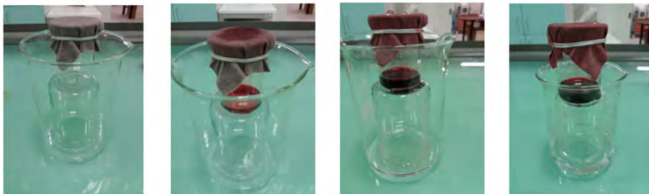
Figure 1. Oil/water separation performance of fly ash/OTMS coated cotton fabrics
