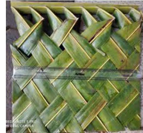
Fig.2 30cm x 30cm coconut leaf for testing
