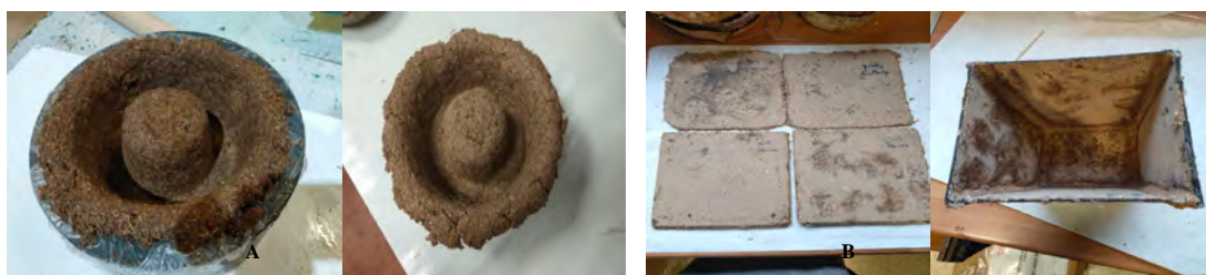
Figure 1: Result of the retainers. A) Wet moulding B) Flat moulding
