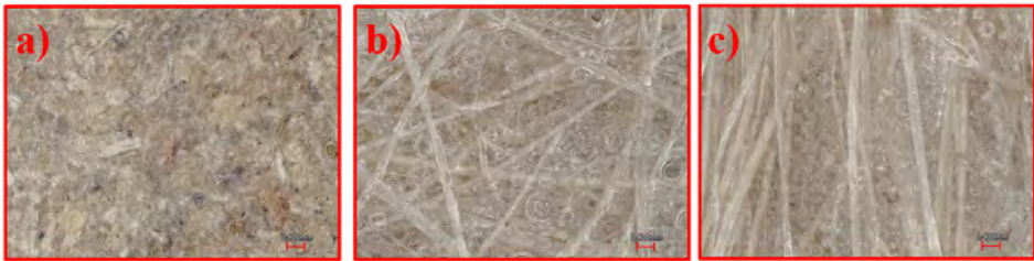
Fig.1 The biocomposites made from epoxy resin and a) fique powder, b) industrial nonwoven Fique Fiber mat and c) unidirectional fique fiber mat
