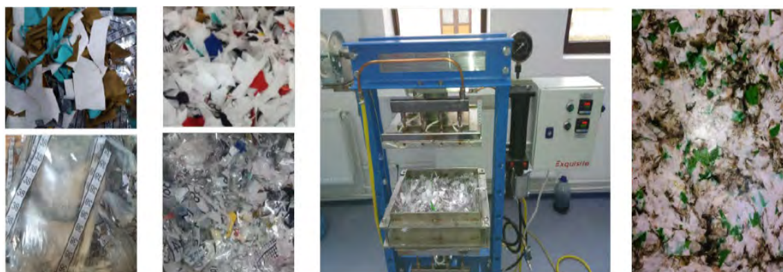
Fig.1 Technological process for producing waste-based composite material
