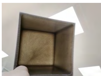
Figure 2. Distribution of ignimbrite powder in the composite parts.
