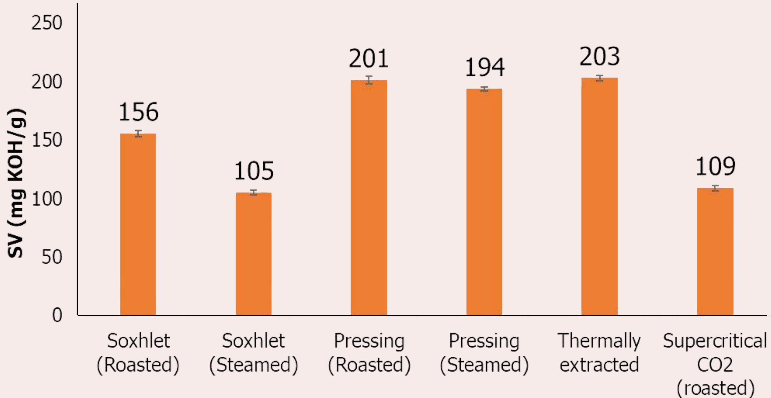
Fig 2. CNSL Saponification value vs Extraction methods
